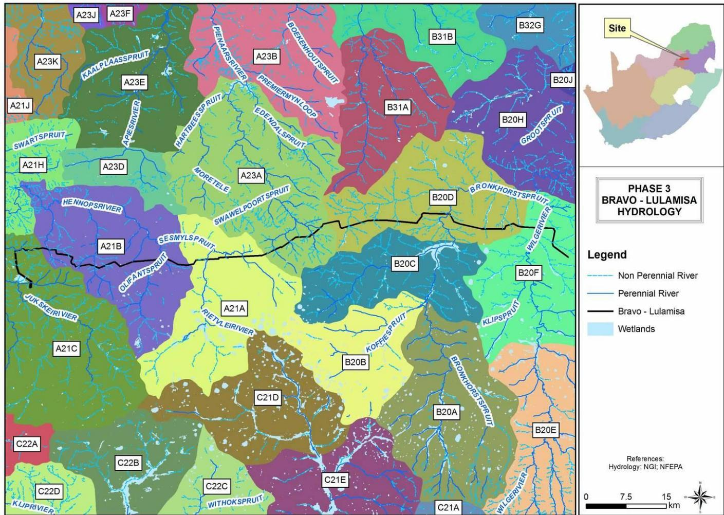
Figure 2: Hydrological data for the proposed powerline. Note that drainage is mainly northwards.
